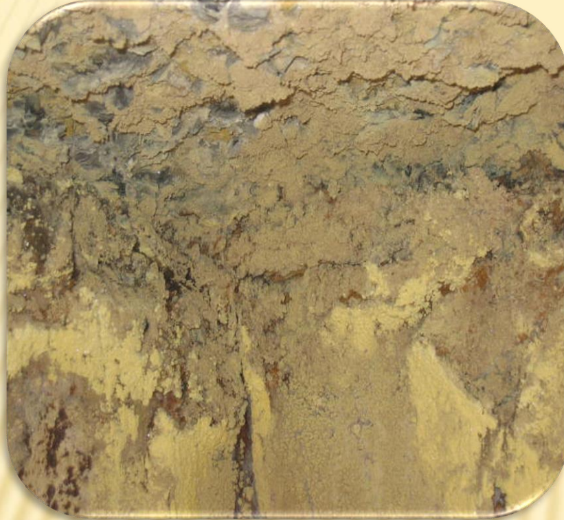
Microbial Induced Corrosion (MIC)
